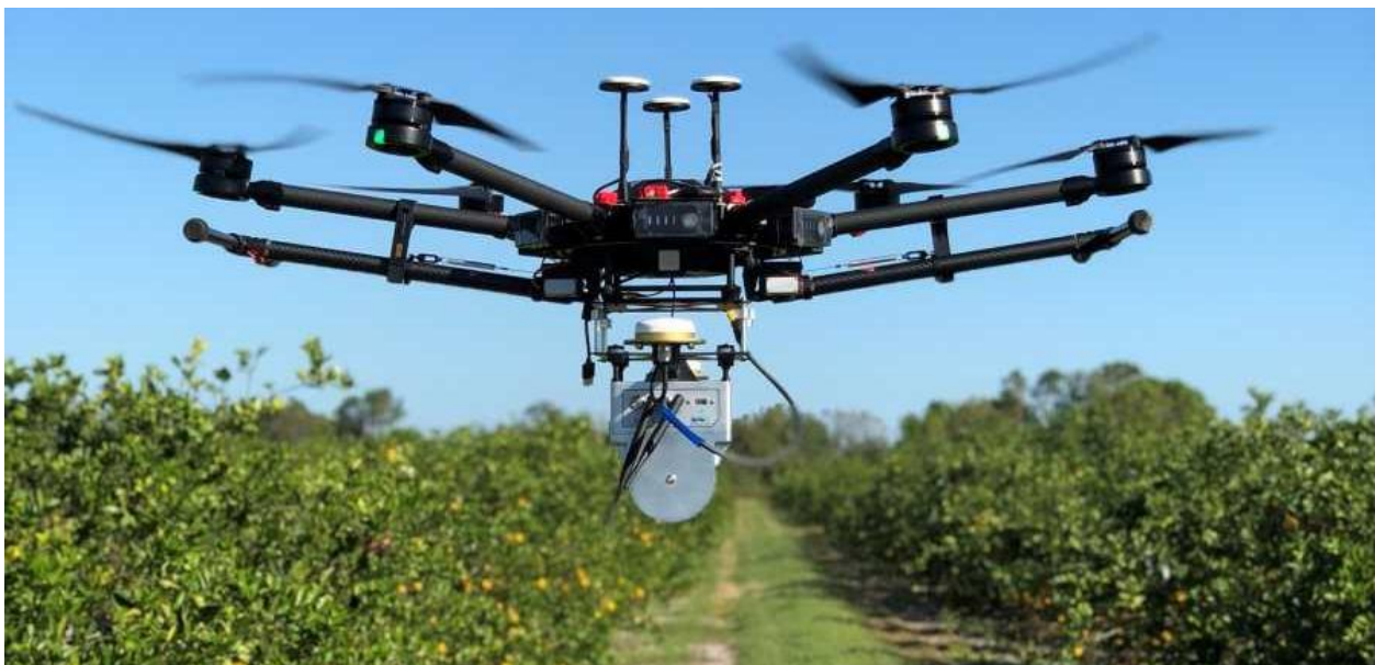
Image: Agricultural drone equipped with LIDAR, photo courtesy of UF/IFAS
